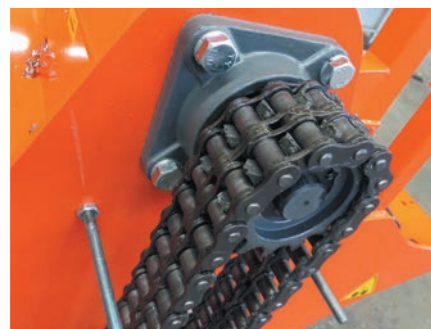
Mechanical drive via duplex chain
