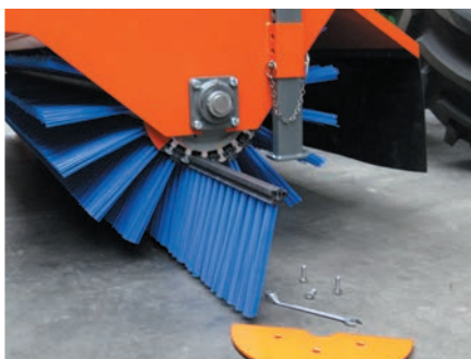
Cartridge system with brush elements
