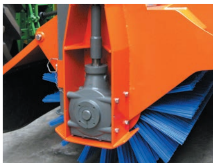
Gearbox (on the side)
