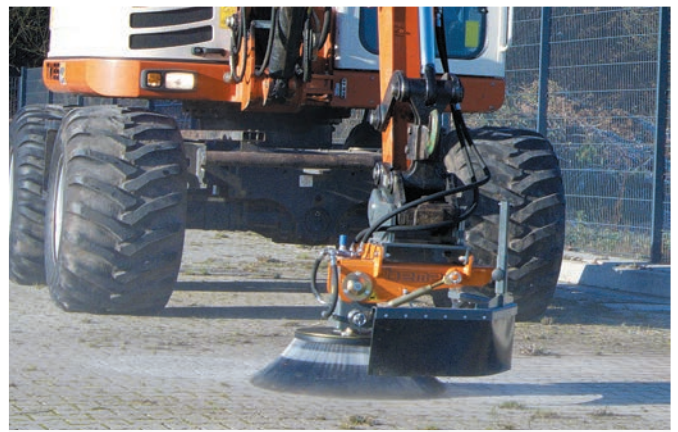
bema Groby optional with an excavator mounting
