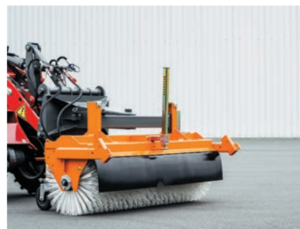
bema 20 without collection container (free sweeping)
