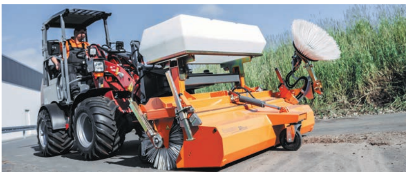
bema 20 Dual with water spray unit and rotary side brush
