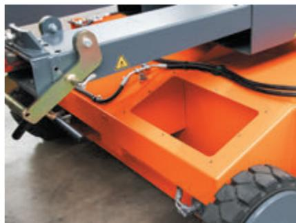
Machine casing with integrated water tank
