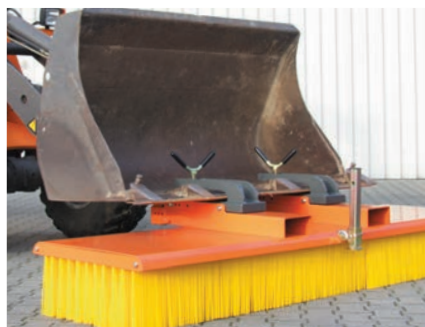
Shovel mounting incl. clamping screws
