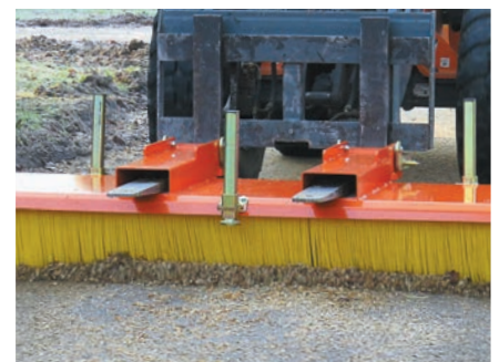
Pallet mounting with a tool-free locking
