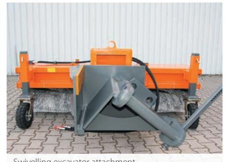
Swivelling excavator attachment (special attachment)
