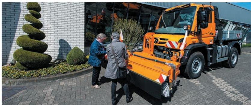
bema 3 Robust with hydraulic lateral movement, attachment for Unimog truck
